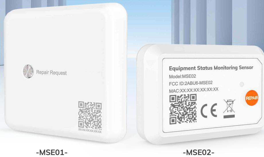
The MSE01 and MSE02 Equipment Status Monitoring Sensors are revolutionary devices that detect device operational states (Off, Standby, or Running) simply by attaching them to the device's exterior-without the need for any circuit connections.
